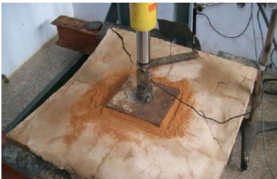
**Figura 38.** Falla probeta B1
