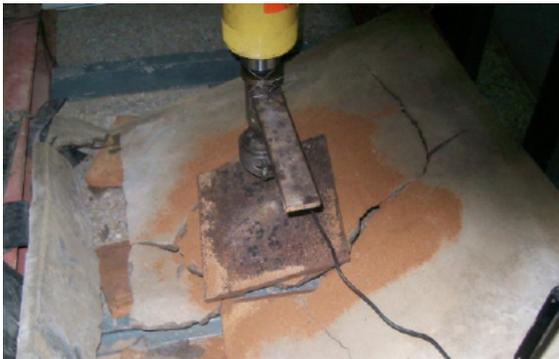
**Figura 36.** Falla probeta A3
